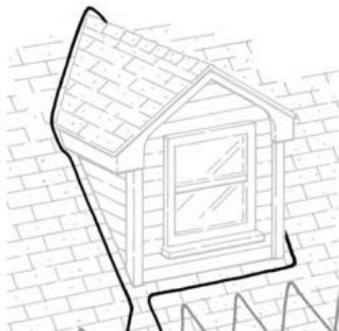
Figure 7. Cable pattern around a dormer
